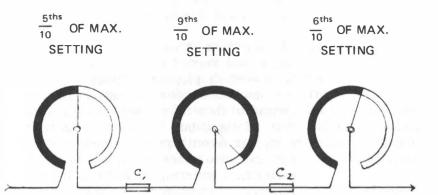
(The capacitors,  $C_1 - C_2$  — or some other method, between the adjustable scales, which are frequently radio potentiometers, serve to prevent the lengths of the connecting wires becoming part of the proportion).
